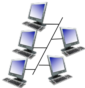
shared wire (e.g., cabled Ethernet)
